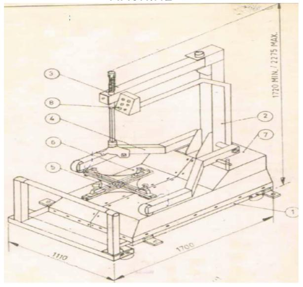
An electro-pneumatic Tyre changing machine designed specially for rear tyre of tractors with proven efficiency at numerous tractor plants across India for fitment and removal of tyres in the fastest possible time. Appropriate for 36" Rim size tyre.
